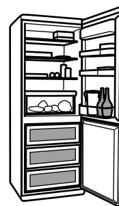
fridge-freezer on for 12 hours during the day and 12 hours at night current of 1.8 amps
